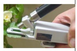
The Standard PAR Clip is designed for one hand operation. The underside opening mechanism prevents the weight of the fibre optic cable opening the PAR clip unexpectedly.
