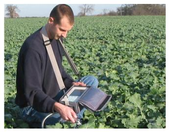
excitation light. The fluorescence intensity is measured and plotted against time. The sophisticated detection system distinguishes between the pulsed response and the non-pulsed response allowing both ambient light and dark adapted experiments to be performed.
